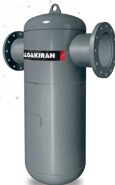
Dalgakiran water separators are designed to remove liquid water and some particulates in compressed air at the compressor outlet. Their unique centrifugal effect separates heavier-than-air matter and the low pressure drop makes them energy-efficient.
