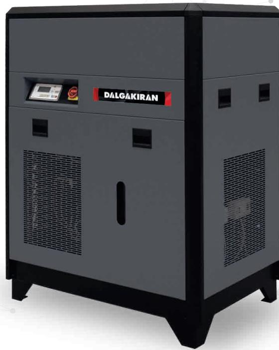
These types of dryers consume energy dependent on air flow. The dryer's cooling system cools the water-glycol mixture down to 1°C and holds this mixture in a stainless steel container. A small pump circulates the water-glycol mixture to cool the compressed air. The cooling system's compressor turns off when the mixture reaches the required temperature resulting in considerable energy savings.
