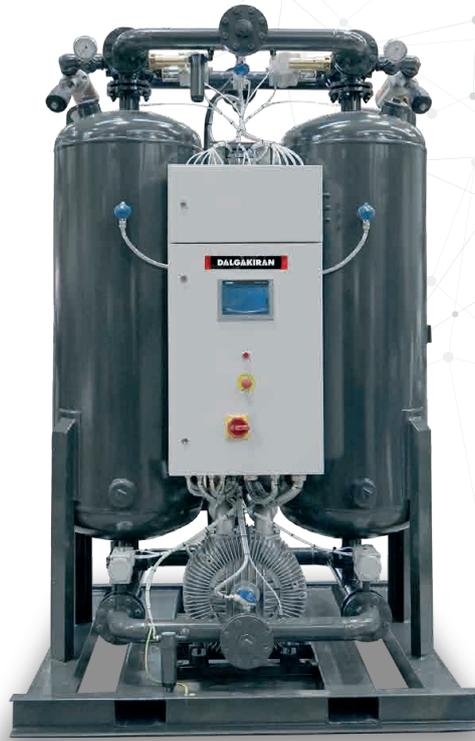
They use a blower to draw in the ambient air and pass it through a heater. The heated air is sent in the opposite direction to the drying flow. This removes the moisture from the chemical substance pores. The advanced control system continuously monitors dew point and adjusts the temperature. This results in energy savings. The heater is insulated for high energy efficiency.
